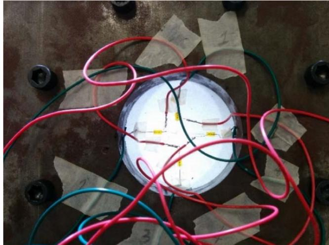
Figure 3. Upper surface of the Mylar sample showing attached strain gages.
